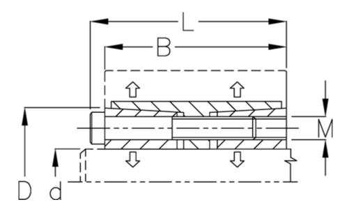
B mm = 105d H8 mm = 200D mm = 260Fit tolerance = Aksel h8, Nav H8
